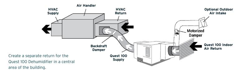
Installing the supply air from the Quest 100 Dehumidifier to the return of the HVAC system requires the HVAC fan to run when the Quest Dehumidifier is operating.
