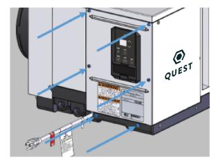
3. Use T25 Torx driver to remove screw from electrical box cover and remove cover.
