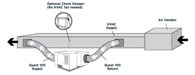
**WARNING!** Due to pressure resistance it is not recommended to use the optional outdoor air intake when installing the dehumidifier supply to supply.
