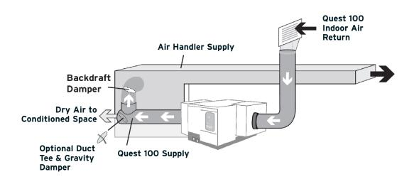
CAUTION! PLEASE NOTE: Return to Return installs are to be considered last resort options and are not recommended. The dehumidifier will heat the AC cooling coils which diminishes the amount of water the AC system will remove when operating. If this installation is chosen, the dehumidifier must activate the HVAC blower and AC calls need to lock out the dehumidifier from running. Please check your local codes prior to installing.
