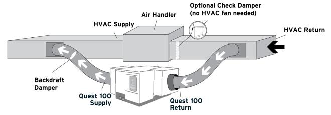
Check Damper should be in place between the Return and Supply connections of the dehumidifier.
