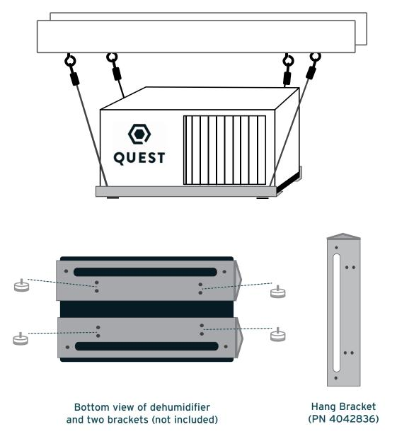
NOTE: LEVELING FEET HOLD BRACKETS IN PLACE
