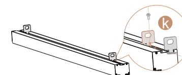
Attach the carabiner from the steel wire hanger to the light bar hole (A). Hang the fixture in your hanging support frame (B).
