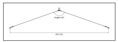
5. Please ensure that the angle is no more than  $140^{\circ}$  and that the distance between the two Eye Plates is no greater than  $94^{\circ}$ .
