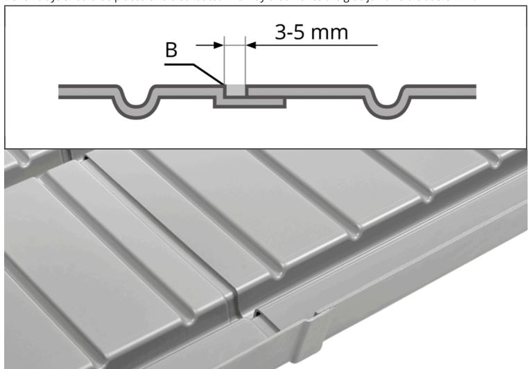
Due to variations in temperature the bench trays work lengthwise. It is therefore important to ensure that there is distance between the edge of the trays and the edge of the bench frames.
